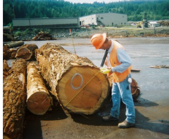
Scalers assess each log, then enter data on dimensions, defects and other criteria using the Ranger handheld.
