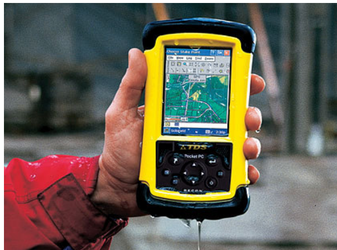
TDS Recon, a ruggedized Pocket PC, being used in the rain
