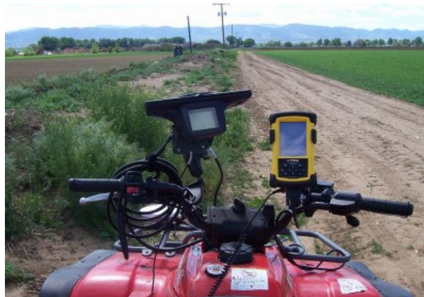
This ATV, equipped with a rugged TDS Recon handheld computer and Trimble AgGPS EZ Map software, is ready to help pinpoint and record weed problems.
